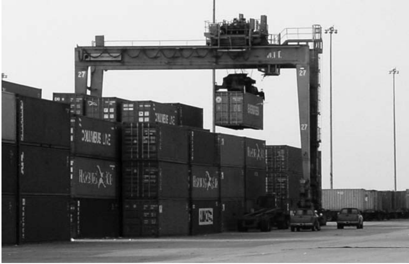
Figure 3.5 Yard gantry crane
