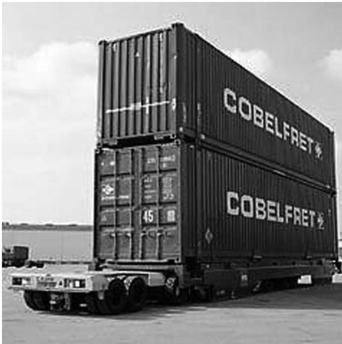
Figure 3.7 Cassette AGV that is double-stacked loaded onto a cassette and transported by an AGV
