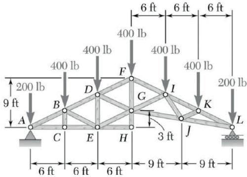
Determine the force in each of the members located to the left of line  $FGH$  for the studio roof truss shown. State whether each member is in tension or compression.
