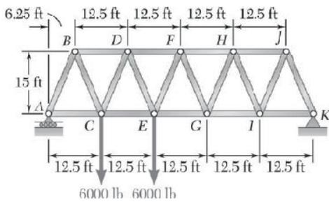
A Warren bridge truss is loaded as shown. Determine the force in members  $CE$ ,  $DE$ , and  $DF$ .
