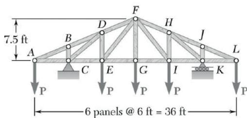
Determine the force in members  $EG$  and  $EF$  of the truss shown when  $P = 20$  kips.
